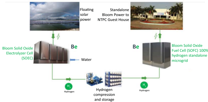
Figure 2: Floating solar park to produce green hydrogen [2]
